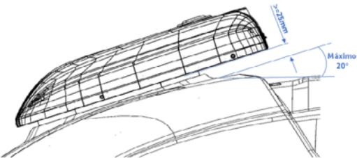
**1.0:** There must be a minimum distance of 25mm between the base of the AC and the surface of the ceiling so that air can enter the condenser without losing flow.
